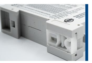
The top hat rail enables quick and easy mounting of the switch in the existing control cabinet. The speed monitor is first placed on the top hat rail with the mounting edge and then pressed onto the top hat rail until the catch engages.
